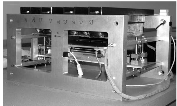
Fig. 1. 2-DOF magnetic levitation hardware implementation
