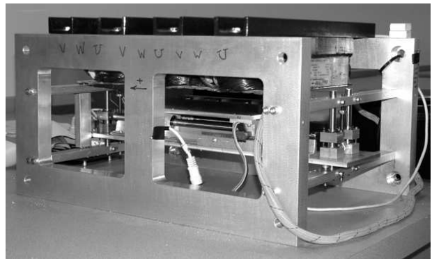
Fig. 1. 2-DOF magnetic levitation hardware implementation
