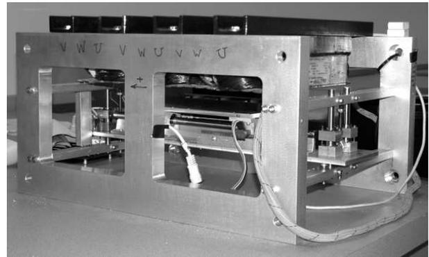
Fig. 1. 2-DOF magnetic levitation hardware implementation
